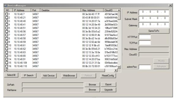
2) Modify the network parameters: select a device, in the action bar on the right can modify the network parameters of the IP address, subnet mask, default gateway, HTTP port, TCP port, then the network parameters of the device modified successfully; click on the "consistent with the local PC" can make the subnet mask and default gateway fit to the PC.
